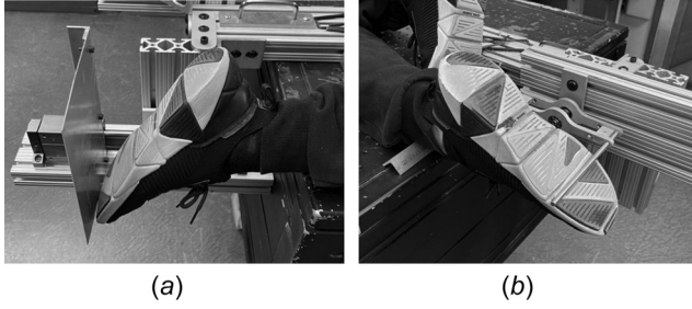
Fig. 5 (a) Linear prototype which incorporates a linear bushing slider and (b) rotational prototype which uses a fixed pivot point
